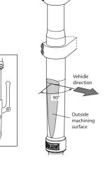
Tighten the triple clamp screws to torque according to the vehicle service manual.
